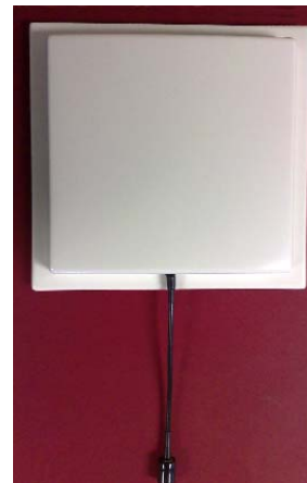
Front View of antenna showing coaxial cable and N-type Connector
