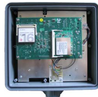
Enclosure with Pc-Engines WRAP Board
