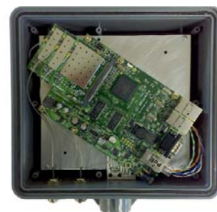
Enclosure with Mikrotik Routerboard
