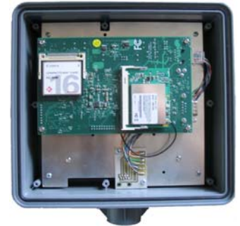
Enclosure with Pc-Engines WRAP Board
