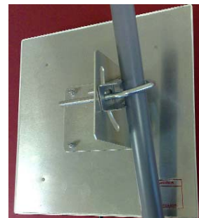
Pole mount tilting bracket fitted to antenna
