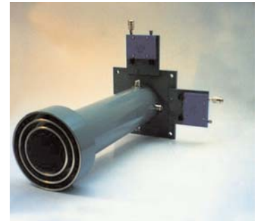
Choked probe view, showing the hybrid feed network
